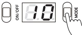
Press the MODE button for 6 seconds until the display shows **b0** or **b1**.
