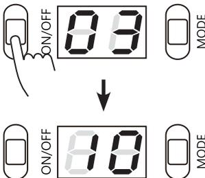
During the exposure time, the operator can push the ON/OFF button to turn off the light. Then the system will generate one beep and reset the time automatically.
