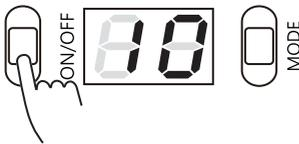
When LEDEX™ WL-070 hand piece is turned on, push the ON/OFF button again to output the light. Final countdown will be showed on the display.
