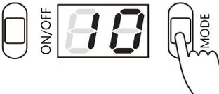
Push the MODE button, the time would be changed as followed 10 secs → 20 secs → 30 secs → 40 secs → 10 secs → 20 secs...
