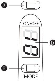
**a** ON/OFF : Press this button start the handpiece. Press this button again to turn on the curing light. Pressing this button during the curing cycle will interrupt and end the cycle. If the unit is in sleep mode, press this button will wake the unit and it will display with the last mode choosen.
