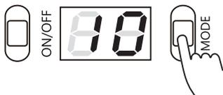
a). Push and hold the MODE button for more than 4 seconds.
