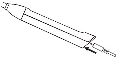
Connect the power supply to AC100~240 V electronic socket and plug-in the connector to LEDEX™ WL-070 hand piece. Push the ON/OFF button to turn on the LEDEX™ WL-070 hand piece.
