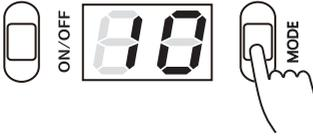
a). Press and hold the MODE button more than 6 seconds. And hear two beeps.
