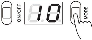
Press and hold the mode button for three seconds. Start to revise the modes after one beep.
