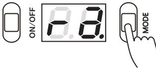
Press the mode button, it will switch to ramp mode, operation panel will display **r.2**
