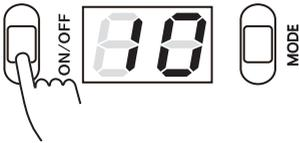
When the status of LEDEX™ WL-070+ hand piece is turning on, push the ON/OFF button again to output the light. Then the display will be showed final countdown.
