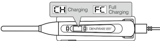
When battery is charged, the display will show CH signal. When battery is full charging, the display will show FC signal.
