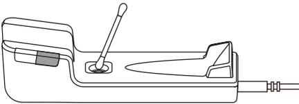
Verify that the radiometer sensor is free of debris that could impact the accuracy of the measurement. If the radiometer sensor requires cleaning.
