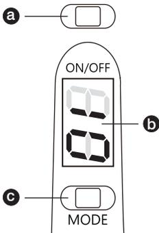
**a** ON-OFF : Pressing this button initiates the selected curing cycles. Pressing this button during the curing cycle will interrupt or end the cycle. If the unit is in the sleep mode, pressing this button will awaken the unit of the curing mode which is last used.
